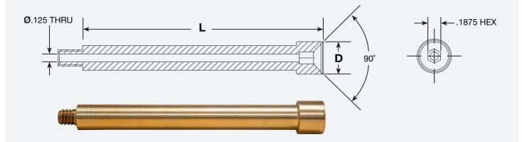
Custom insert lengths and diameters are available on request
