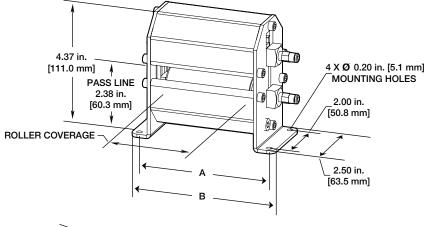
Vertical Mini-Rollers<sup>™</sup> coverage up to 6" [152 mm]
