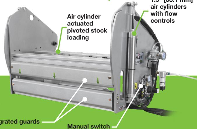
All Uni-Roller® S2 HG lubricators have guards on the entry side only.
