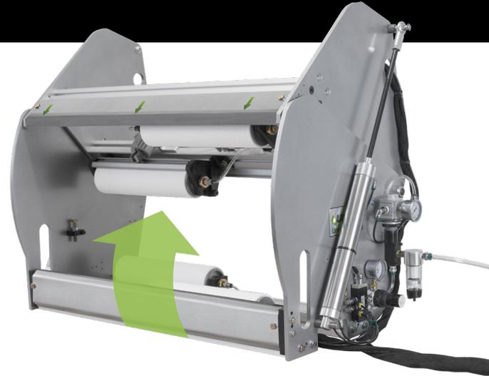
The Uni-Roller® S2 HG is modular in design. Opening and closing is controlled by a manual or solenoid valve. A single roller set is used for widths of 18" [457 mm] or less. For stock over 18" [457 mm] wide, multiple 12" [305 mm] wide roller sets are staggered and overlapped. Standard sizes are available to accommodate common stock widths, with custom sizes available on request.
